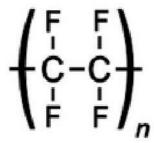
In PTFE, due to large fluorine Atom, PTFE Molecule takes up a twisted zigzag, with the fluorine atoms packing tightly in a spiral around the Carbon-carbon skeleton. This compact interlocking of fluorine atoms lead to a PTFE molecule of great stiffness leading ultimately high crystalline melting point @ 327°C, thermal stability & electrical insulation properties. Due to strong & stable bond between carbon & fluorine atom, PTFE molecule processes outstanding chemical inertness
